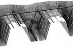
Section through profiled metal of concrete floor.
